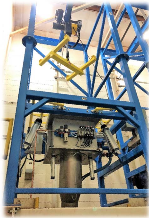
Two Units, Platform Mounted, Through Discharge Tube to Pneumatic Conveyors
